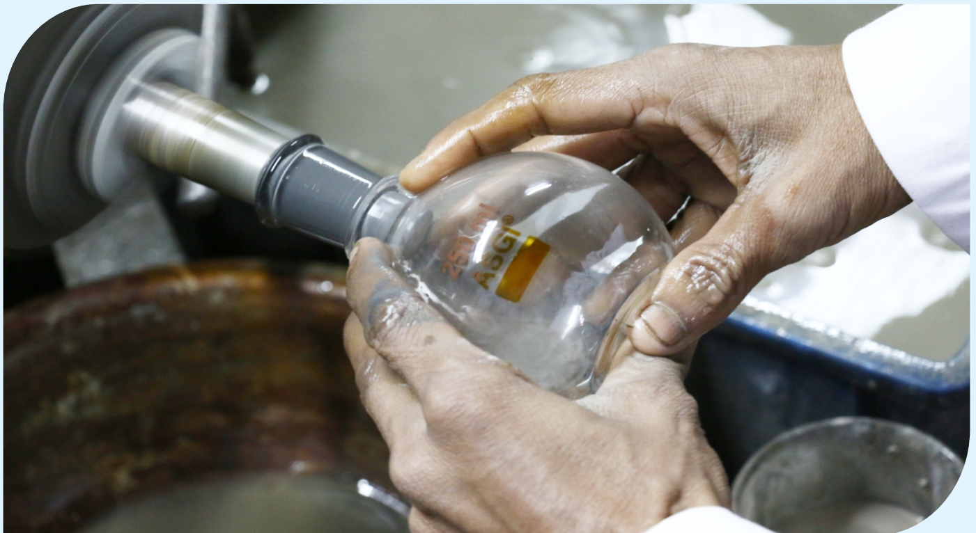
grinding & polishing of joints
