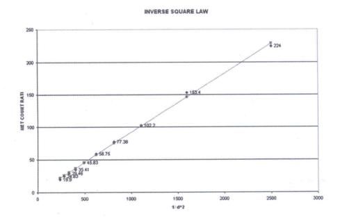
Fig (9). Plot of Net Count Rate (R) Vs Inverse Square of Distance (d)
