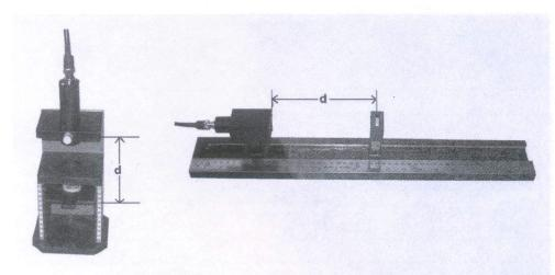
Fig. 7 : Detector, G.M. stand / holder and source arrangement
